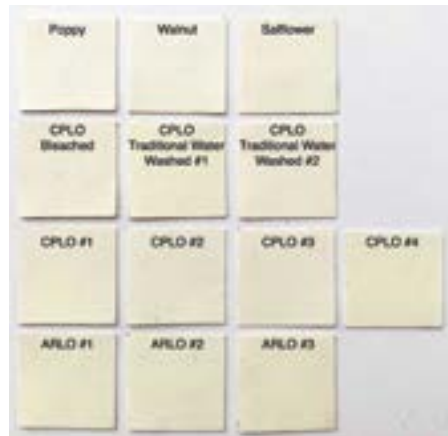
Image 1: One inch square sections of Whatman® filter paper that had 3 drops of oil placed in the center. Three sets using 13 different oils were aged for 2.5 years in room lit with full spectrum fluorescent lights running on alternating 12 hour cycles.
