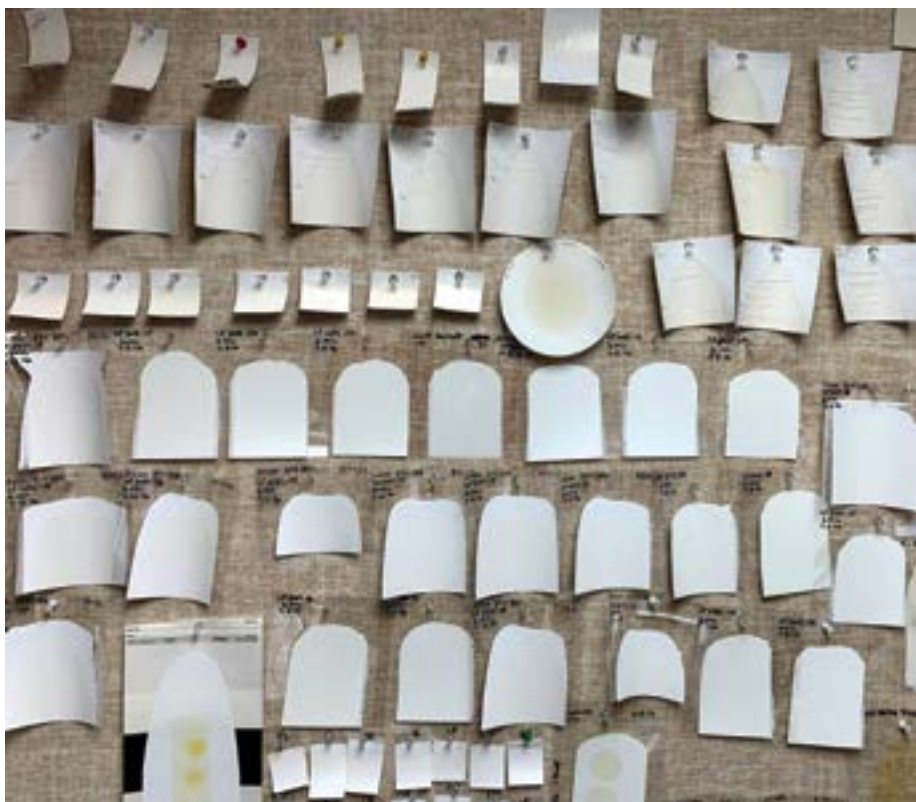
A range of test samples exposed to the typical mix of fluorescent and indirect window light for the last 30 months.
