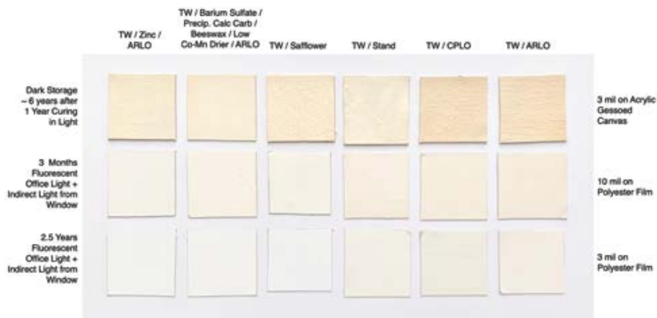
Image 6: All samples cast in 2010. Formulas adjusted so paints had similar viscosity. Samples initially exposed to fluorescent light for first year. Top row were kept in dark storage for ~ 6 years. Middle and Bottom rows exposed to a mix of both fluorescent and indirect window light for 3 months and 2.5 years respectively.
