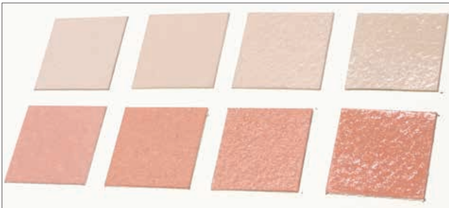
Figure 1: Light and medium washes of QoR Pyrrole Red Light with (left to right) no varnish, 2 layers, 4 layers, and 6 layers of Archival Varnish (Gloss).
