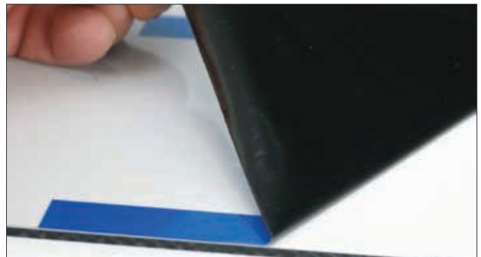
Peeling backer off Dibond®
