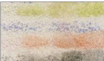
Figure 14: Glass Bead Gel acted like no other media. Color remained in grooves after being wiped.
