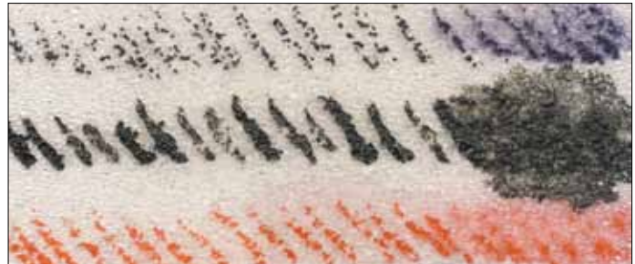
Figure 4: Glass Bead Gel tended to hold wet media within its crevasses while allowing the tops of the glass beads to be wiped clean.
