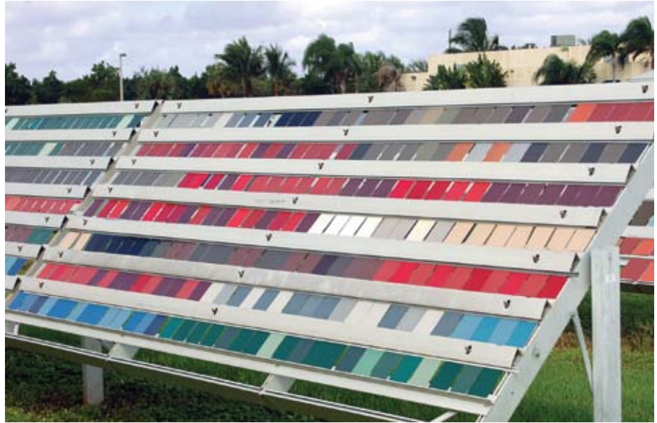
Facility in South Florida testing the OPEN Acrylics at a severe 45 degree angle to the sun. Photo courtesy of Q-Panel.
