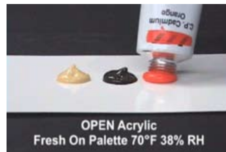
Screen shot from new video demonstrating the open time properties of the new OPEN Acrylics.
