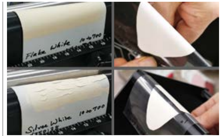
Image 2: All samples are 6 mil drawdowns from 2010-2011. Flake (top left) and Silver White (bottom left) are on aluminum panels bent over a cone. Titanium (top right) and Titanium-Zinc White (bottom right) are on polyester film bent over different diameters of dowels and rolled edges. Flake White showed no cracking, while Silver White, made with Lead and Zinc, showed extreme brittleness. Titanium White, which is zinc free, remained flexible even when bent over 1/8", while Titanium-Zinc cracked easily at 1".
