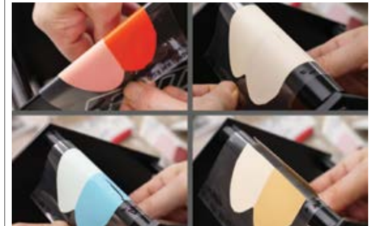
Image 3: All samples are 6 mil drawdowns from 2010 on polyester film and bent over different diameters. Cadmium Red Light (top left), made without zinc, remained extremely flexible and could be easily bent over a 1/8" diameter rolled edge. In contrast, Zinc Buff (top right) started to crack at 1", King's Blue (bottom left) at 5/8", and Naples Yellow Reddish (bottom right) easily snapped in half at 3/4". Both of these blends had zinc in them.
