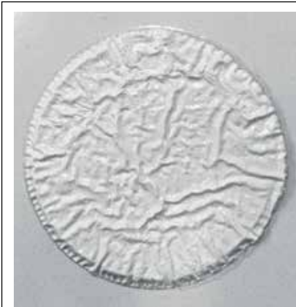
Figure 6: 60 mil test sample of titanium dioxide ground in alkali-refined linseed oil.
