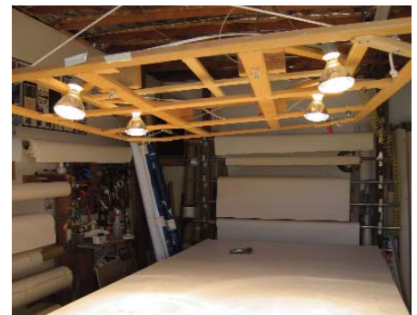
A home-made overhead frame with infrared heat lamps may be raised and lowered via pulleys. Warming pre-primed canvas makes it supple and much easier to stretch. (Courtesy of John Annesley Co.)
