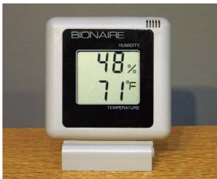
The humidity-temperature gauge clearly reads 48% RH (relative humidity) and 71° F.
