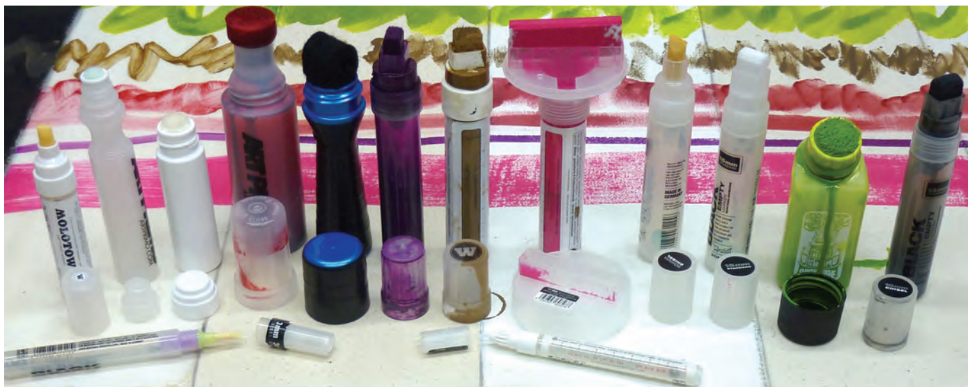
There are a wide variety of markers with varying tips and nibs available. The nib sizes range from .7mm up to 60mm with many sizes in between. We tested tips and nibs in the following sizes: 2mm, 3mm, 5mm, 10mm, 15mm and then 60mm.
